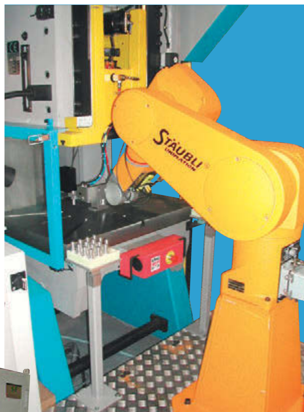
25 T press with automatic robotic loading
